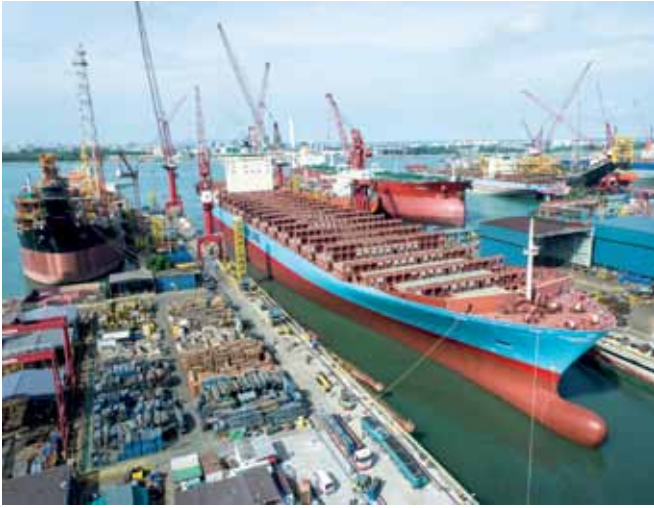
The 366-metre container ship from A.P. Moller-Maersk, Mette Maersk, was the first vessel to benefit from the extension of Raffles Dock to 400 metres
